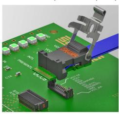
Align optical or copper assembly so that notches in PCB are over the positive latching receptacle.
