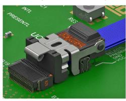
Depress latch to lock cable assembly into the connector.
