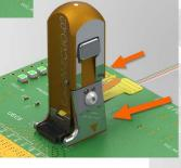
To remove tool press the side button and lean tool slightly to the right and lift tool upwards.
