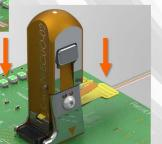
2 Drop tooling with cable assembly down keeping it parallel to board.
