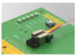
Remove by pulling the latch position retainer.
