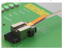
**5** Depress latch to lock cable assembly into the connector.
