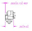
EIG 4 (-K OPTION) BTH-090-01-X-D-RA-WT-MGP-K SHOWN (SAME AS FIG 2, EXCEPT AS SHOWN) (SOME CENTER FEATURES REMOVED FOR CLARITY)
