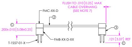
No OF POSITIONS -03 TO -25 **END ASSEMBLY** -D: DOUBLE END -S: SINGLE END \*-T: TRANSFER END ASSEMBLY LENGTH (2.00[50.8] MINIMUM) LEAD STYLE **PLATING OPTIONS LEAVE BLANK FOR STANDARD** (USE T-1S57-01-T AND C-67-L) L: SELECTIVE LIGHT GOLD
