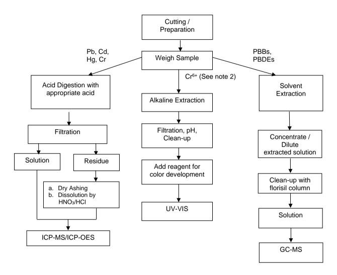
The Cd, Pb, Hg contents test on polymeric samples were dissolved totally by pre-Note conditioning method according to above flow chart.
