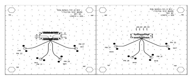
PCB-102944 -TST-03 Rev, FS5 Floating Socket *mates with* PCB-102944 -TST-13, Rev, FT5 Terminal, <u>Differential Best Case Configuration</u>, Transmission/Reflection Parameters, Crosstalk Parameters, Via Location: Outboard
