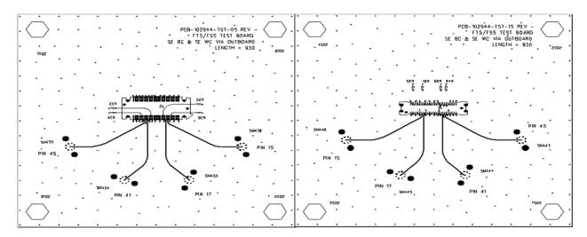
PCB-102944 -TST-02 Rev, FS5 Floating Socket *mates with* PCB-102944 -TST-12, Rev, FT5 Terminal, <u>Single-Ended Best & Worst Case Configurations</u>, Transmission/ Reflection Parameters, Crosstalk Parameters, Via Location: Inboard
