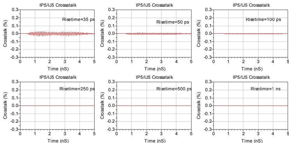
**Series:** IJ5/IP5**Description:** IsoRate, 4.0mm (.157") Pitch, 10mm (.397") Stack Height**Single-Ended Application – NEXT, “4-1” Configuration**
