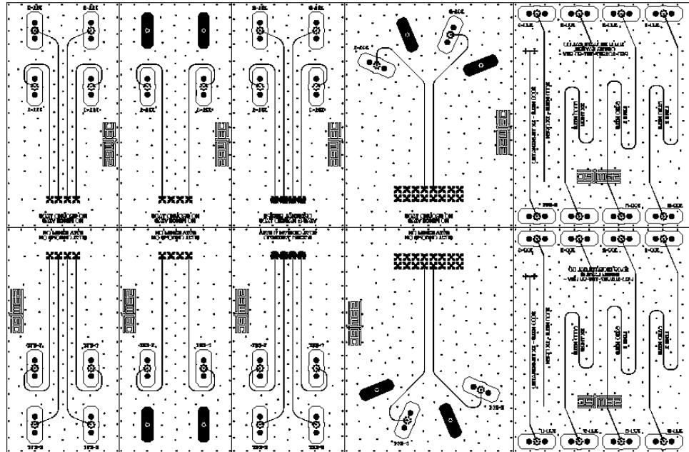
**Series:** IJ5/IP5**Description:** IsoRate, 4.0mm (.157") Pitch, 10mm (.397") Stack Height**PCB Fixture Set I**
