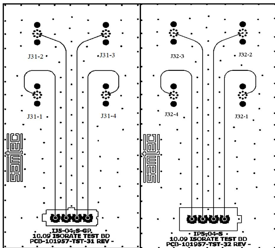
**Series:** IJ5/IP5**Description:** IsoRate, 4.0mm (.157") Pitch, 10mm (.397") Stack Height**Calibration Board**
