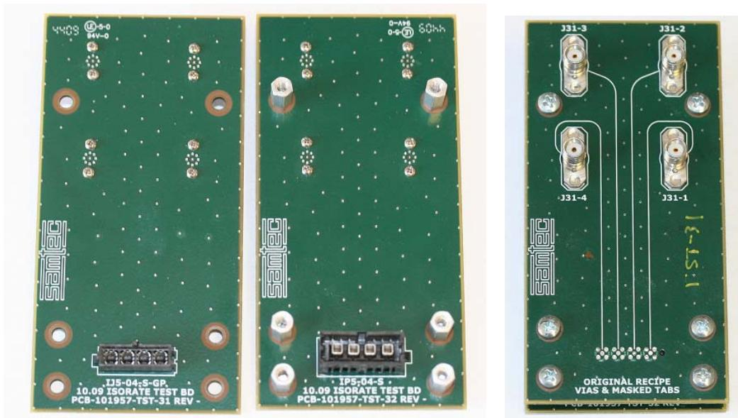
**Series:** IJ5/IP5**Description:** IsoRate, 4.0mm (.157") Pitch, 10mm (.397") Stack Height**PCB-101957-TST PCB Layout Panel**
