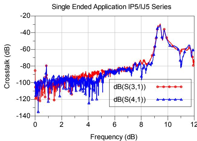
**Series:** IJ5/IP5**Description:** IsoRate, 4.0mm (.157") Pitch, 10mm (.397") Stack Height**Single-Ended Application – NEXT and FEXT, “4-1” Configuration**
