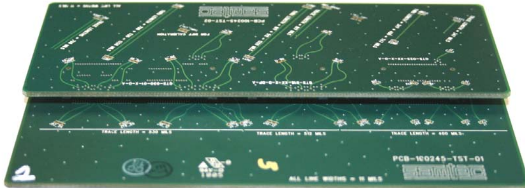
Figure 1 Mated PCB Test Fixture with Mounted Test Connectors
