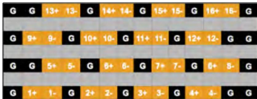
**Figure 13 - High Isolation Differential Vertical**
