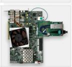
FMC+ HSPC Loopback Card Supports AMD Virtex® UltraScale™+ VCU118 Kit
