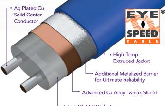
Low Dk FEP Dielectric Co-extruded Technology for World Class Dimensional Consistency
