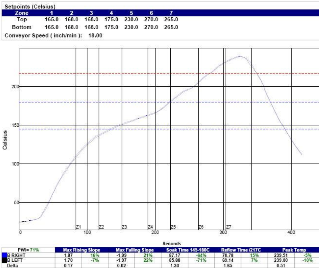
Fig. 9. Example of Lead-Free (Sn96.5 Ag 3.0 Cu 0.5) – Traditional Soak
