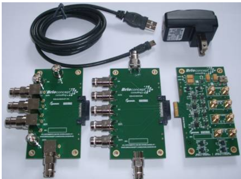
Figure 1. 3G SDI Demonstration Board
