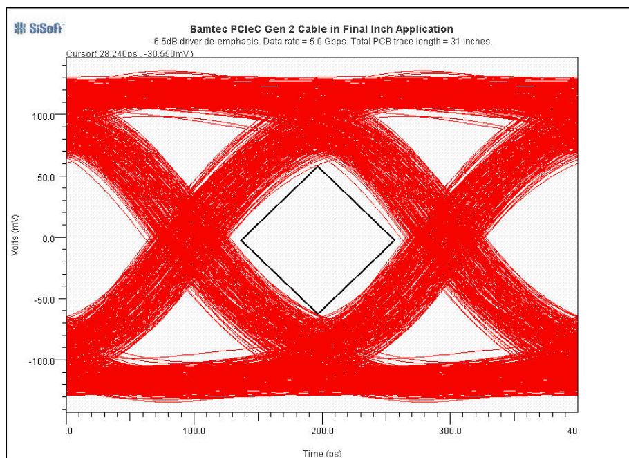
Picture 7 – Receiver eye measurement, probed at far end termination. Standard driver setting with - 6.5 dB de-emphasis. Total trace length = 31 inches.
