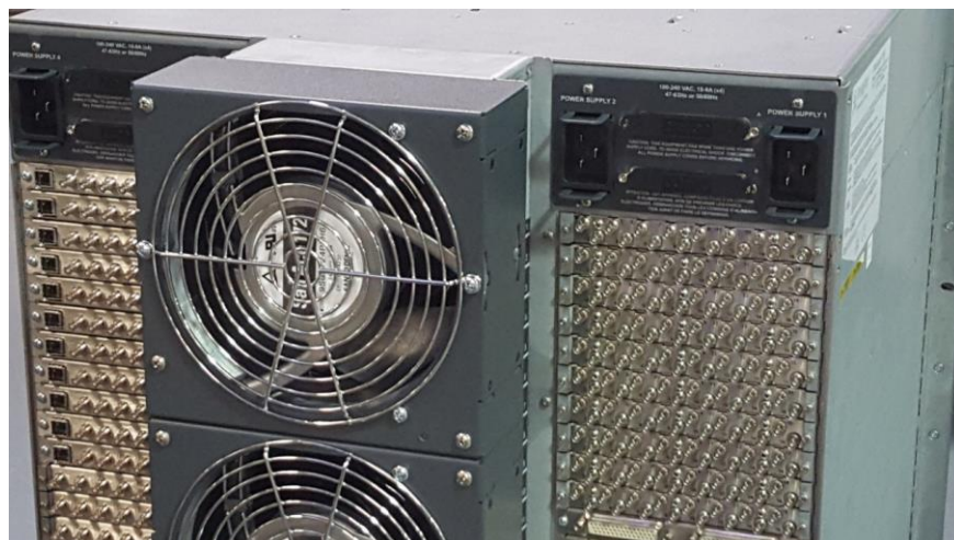
Figure 1. Broadcast Video Equipment Port Density (Courtesy of Imagine Communications)
