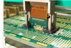
Blind mate transceiver connector (source: Samtec)
