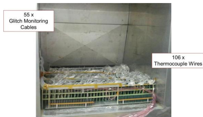
Figure 10: Thermal Cycling Test Vehicles with Cables and Thermocouples Attached
