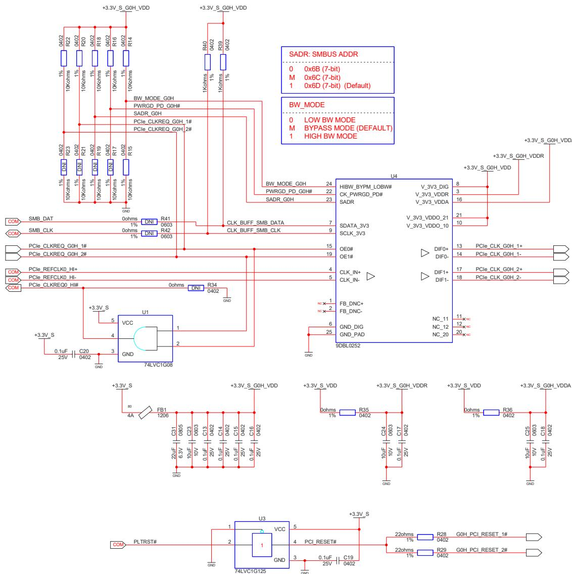
A dual channel clock buffer is used as there are two PCIe x4 links implemented in this PCIe Group 0 High example. The COM-HPC PCIe\_CLKREQ0\_HI# signal is driven by logic gate U1 in the Figure just above, resulting in a clock request if either one or both of the NVMe cards are present. Alternatively, U1 could be removed and the COM-HPC Group 0 High clock request line held low by R34, in which case the Group 0 High PCIe clock pair would always run.
