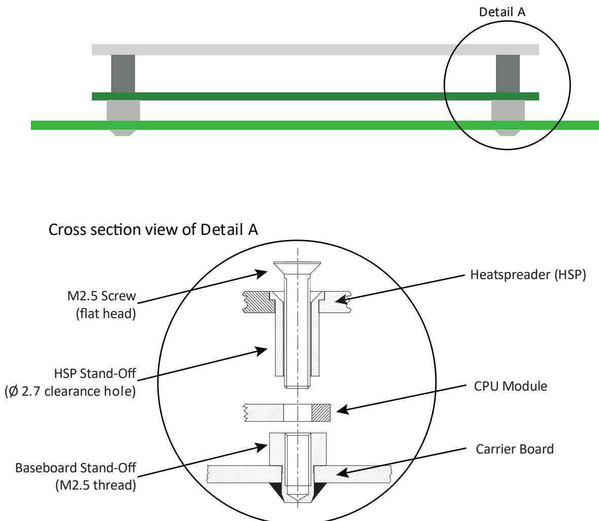
Figure 65: Heat Spreader Assembly Mounting to Carrier With Broaching Nut – Top Side Screw Access
