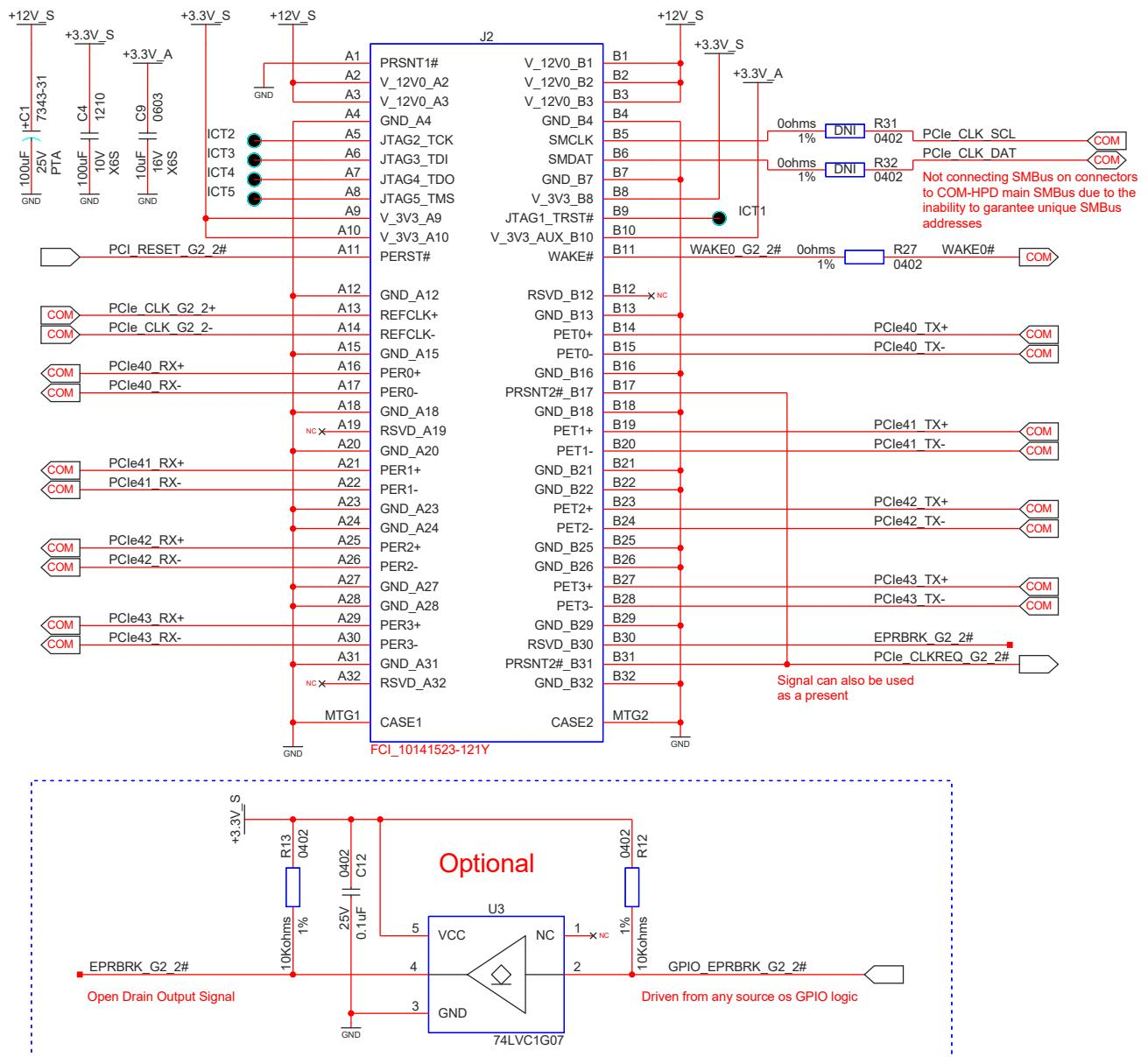
**Figure 23: PCIe x4 Slot Card Site on PCIe Group 2 PCIe Lanes 44:47**
