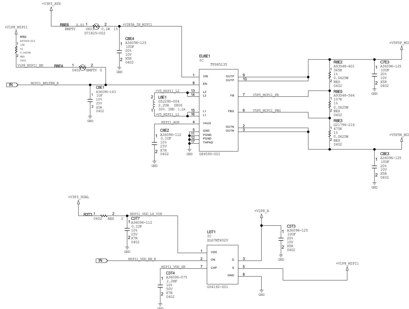
**Figure 81: Alternative eDP Example (Sheet 6 of 6): High Side Gate Driver for eDP Backlight**
