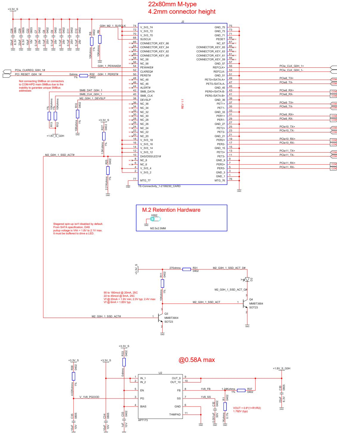
**Figure 18: M.2 M -Key Site for NVME SSD #2 in Group 0 PCIe Lanes 12:15**
