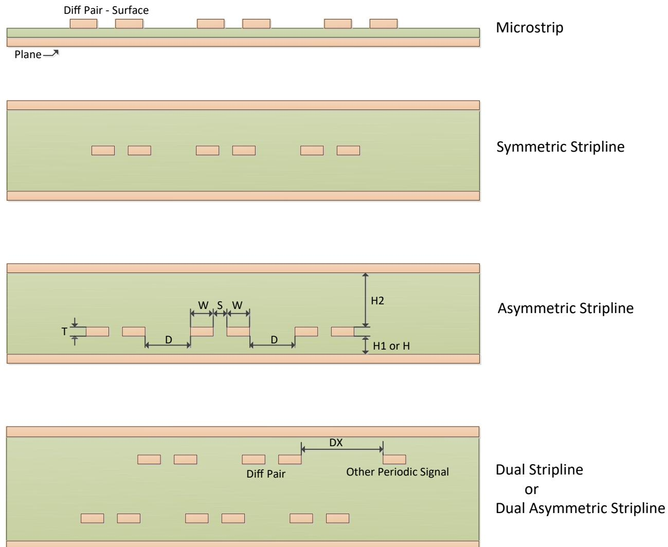
Some of the terms and notations in the Figure above are used in the Tables and text on the following pages. The long copper colored thin rectangles represent the GND or PWR planes and the smaller rectangles, for the most part, the edge coupled differential pairs. The upper and lower signal layers within a Dual Stripline structure should be routed orthogonally to each other to minimize coupling and thereby crosstalk.
