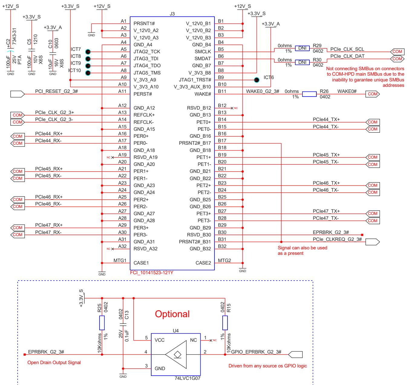
**Figure 24: PCIe Clock Buffer and Reset Buffer for PCIe Group 2 Example**
