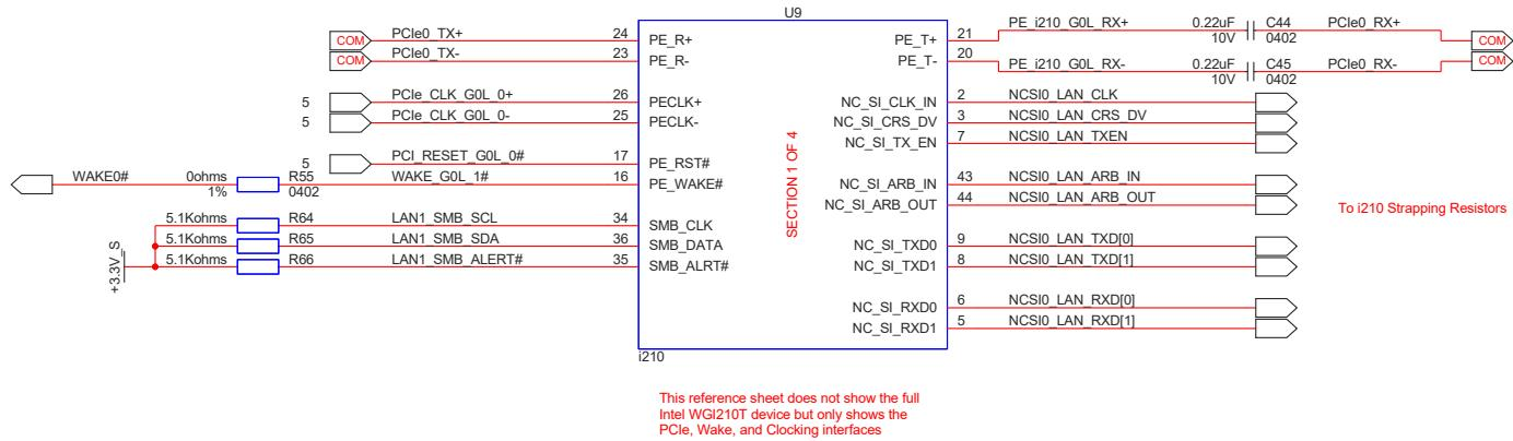
**Figure 13: Mini PCIe Site – PCIe Group 0 Low – PCIe Lane 1**
