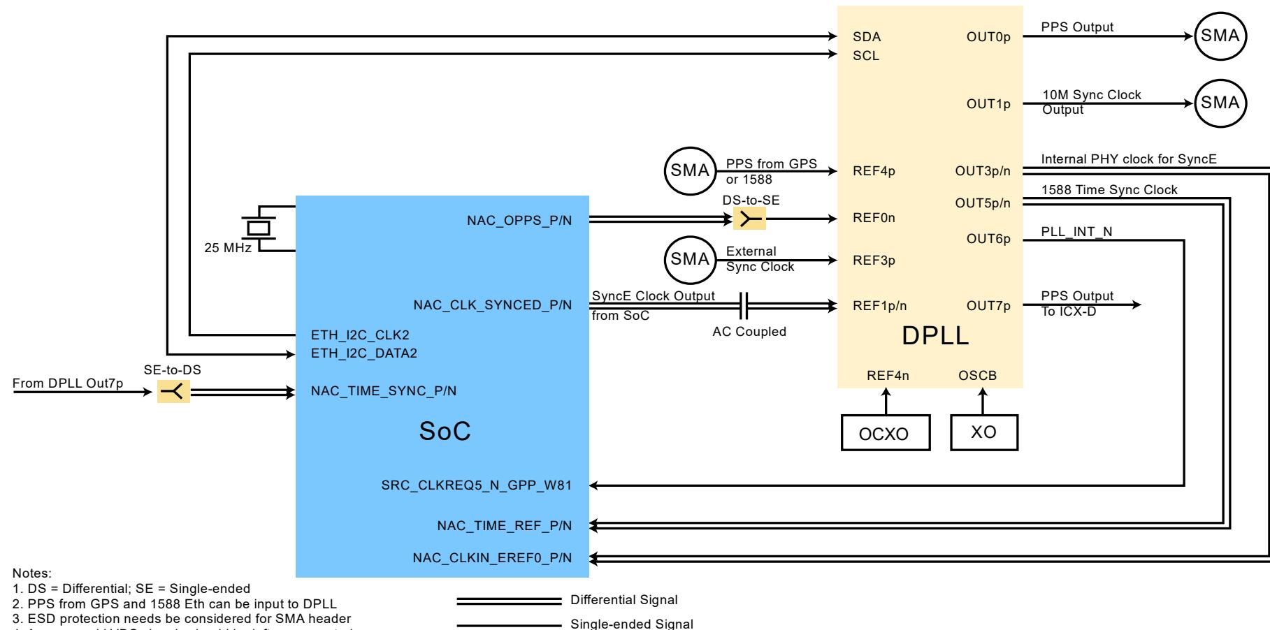
**Figure 75: Synchronous Ethernet Example Implementation**
