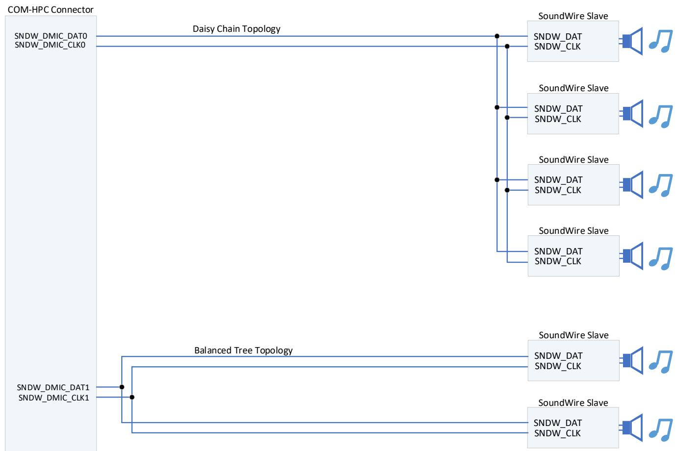
**Figure 51: MIPI SoundWire Point to Point Connection With SI Components**
