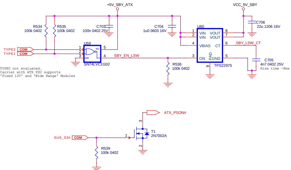
The Carrier hardware shown in Figure 60 below holds off power distribution if the Module Type is not a Server Type Module. The example uses an AT style supply.
