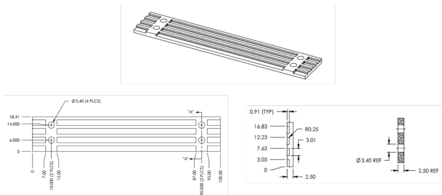
Figure 72: Carrier Board Stiffener Keep-Out Region (Seen Through Carrier)
