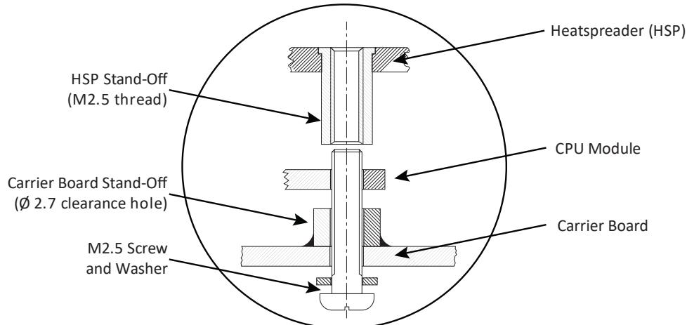
Figure 64: Heat Spreader Assembly Mounting to Carrier – Top Side Screw Access
