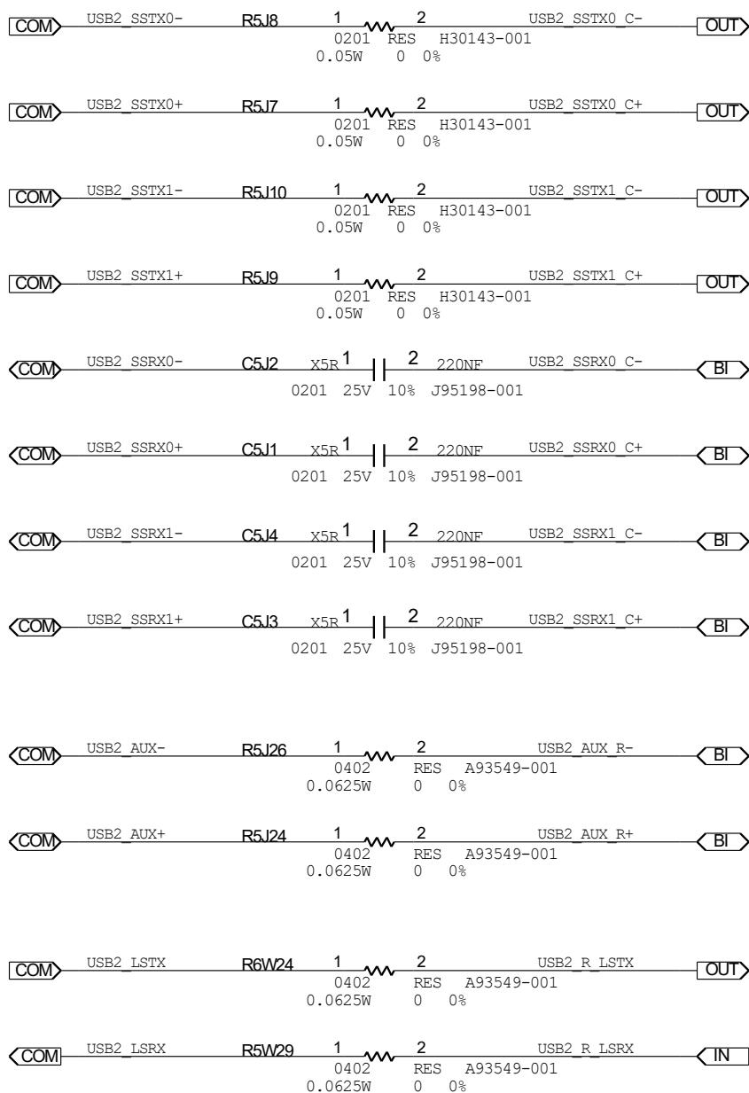
**Figure 37: USB4 on COM-HPC USB Port 2 (Fig 2 of 6): Intel JHL8040R Thunderbolt Retimer Part 1**
