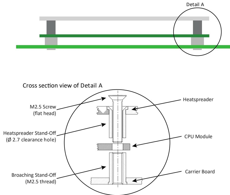
Figure 66: Heat Spreader Assembly Mounting to Carrier and Chassis – Top Side Screw Access
