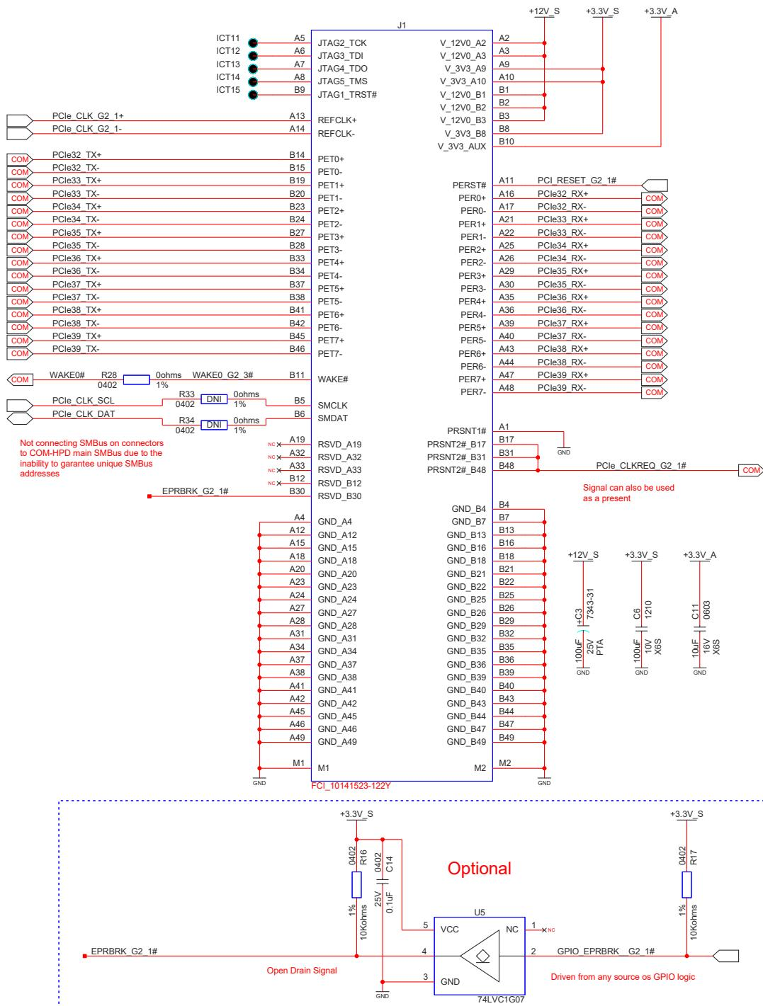
**Figure 22: PCIe x4 Slot Card Site on PCIe Group 2 PCIe Lanes 40:43**
