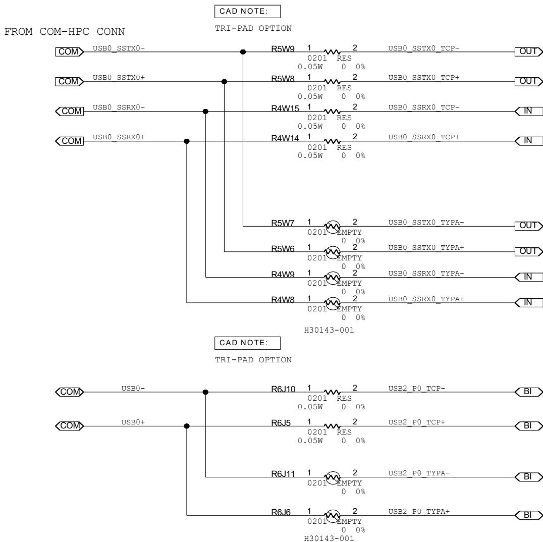
Figure 31: USB 3.2 Gen 2x2 Type-C (2 of 6): Port Multiplexer and Redriver
