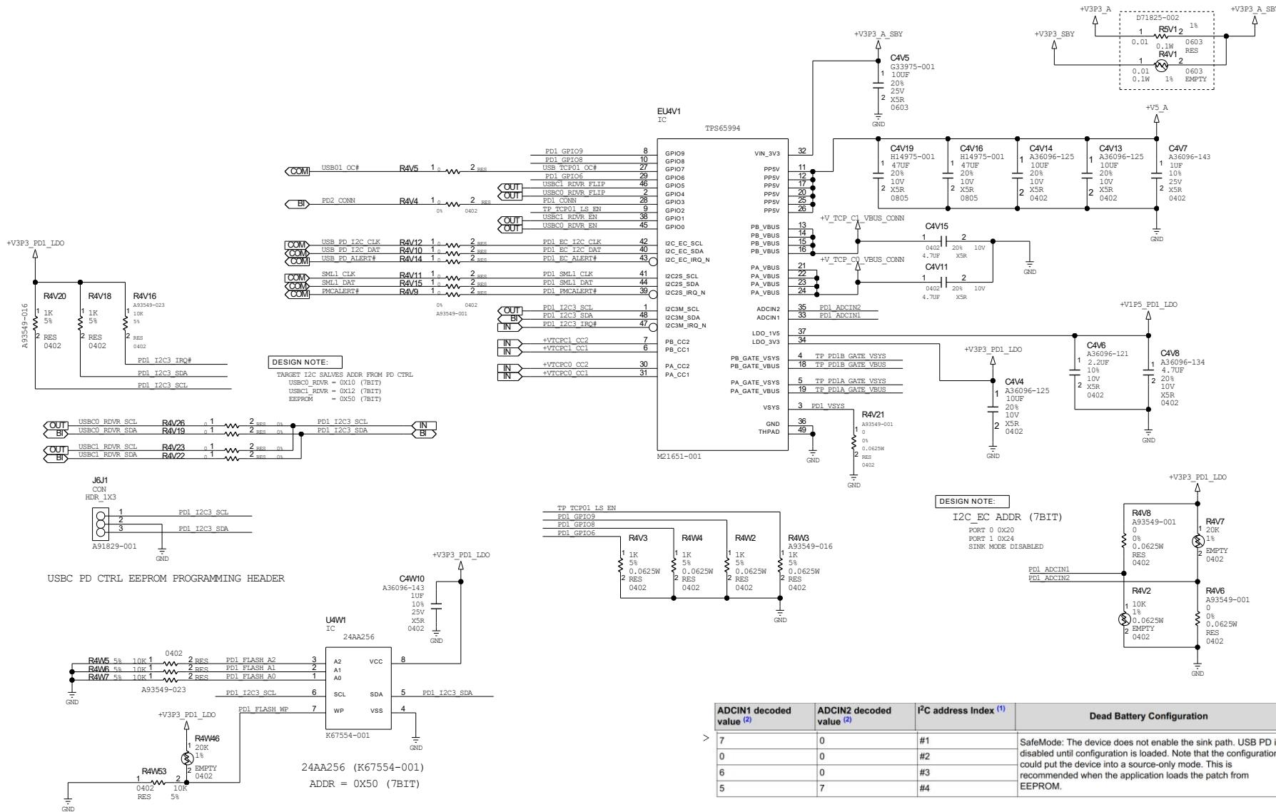
**Figure 35: USB 3.2 Gen 2x2 Type-C (6 of 6): Type-C Connector and Port Protection**
