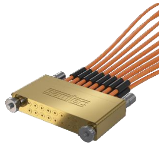
Figure 6: The Samtec BE130 features mode-free performance to 130 GHz and lowest insertion loss and highest frequency possible for 1.0 mm-based equipment. It has an expanded mode-free bandwidth beyond 448 Gbps fundamental frequencies.
