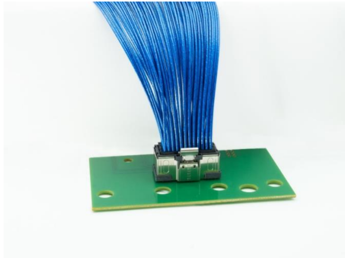
Figure 3: It is best to allow cables to splay to avoid putting stress on the connector.
