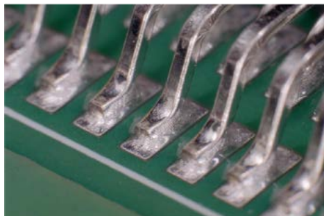
FTSH Samtec Sample 38 0.150 mm (.0059") Coplanarity, 0.10 mm (.004") SP1D Stencil
