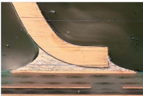
FTSH Samtec Sample 189 (Outer Row) 0.152 mm (.0060") Coplanarity, 0.10 mm (.004") SP1D Stencil
