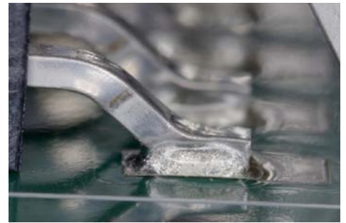
TSM Phoenix Contact Sample (Representative) 0.10 mm (.004") SP1D Stencil
