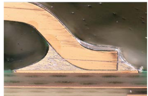
FTSH Samtec Sample 189 (Inner Row) 0.152 mm (.0060") Coplanarity, 0.10 mm (.004") SP1D Stencil
