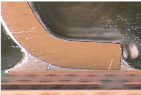
TSM Samtec Sample 3 (Outer Row) 0.160 mm (.0063") Coplanarity, 0.10 mm (.004") SP1D Stencil
