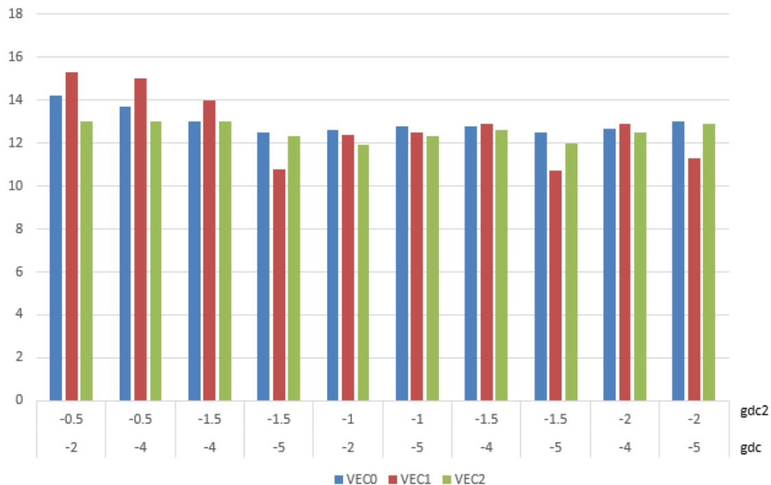
Figure 10. Analysis subset of VEC results while changing the variable CTLE settings (g DC and g DC2 ) during the measurements at TP1.
