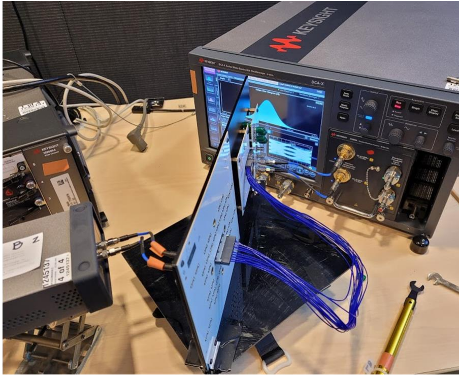
Figure 6. Measurement setup at TP1a: BERT remote Head – 0.15 m instrumentation cable – DUT (based on 12” flyover cable) - 0.15 m instrumentation cable – Oscilloscope.
