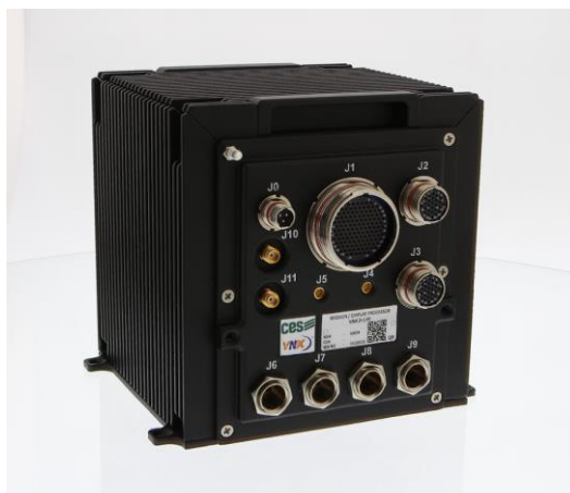
Figure 2: VITA 74 Image Processor With Optical MT Interconnects
