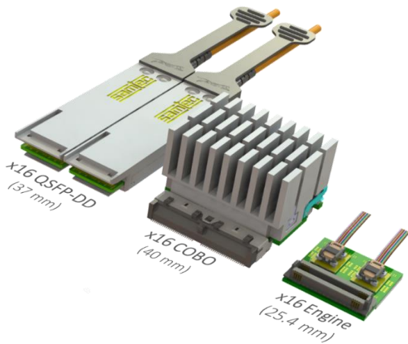
Fig. 8: Size Comparison of a TGV-Based Optical Transceiver Versus Industry Standard.
