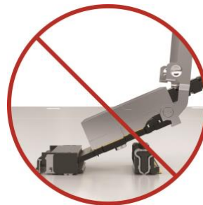
Figure 4. Without Insertion Tool, Bad Insertion Example
