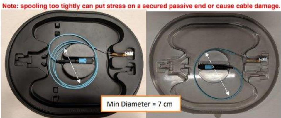
Figure 1. Minimum Bend Radius Example
