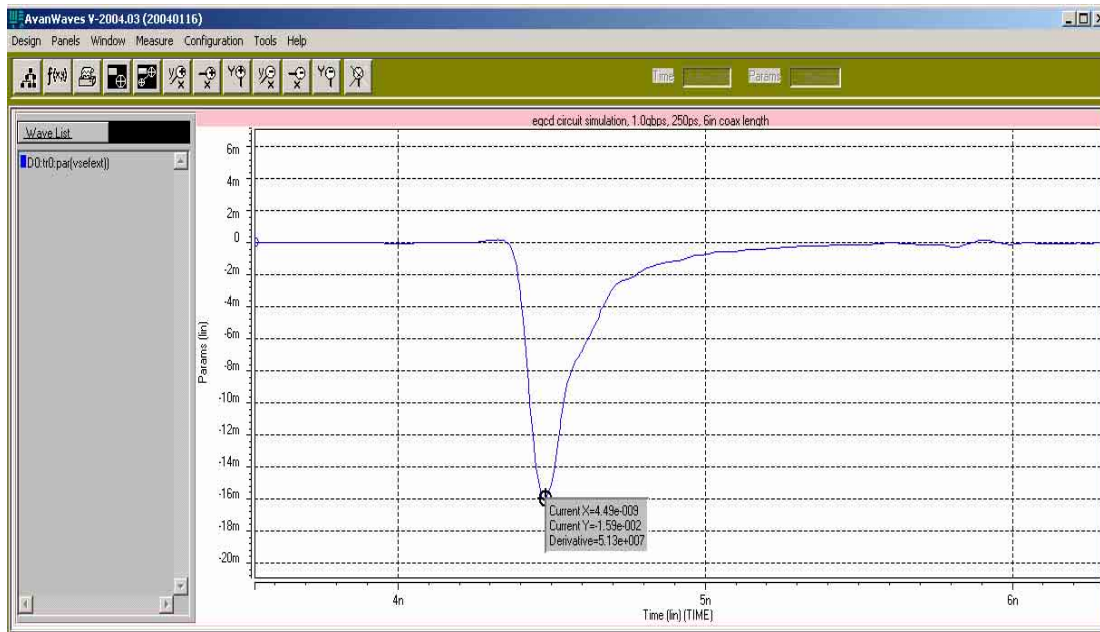
Figure 16: Simulated Far End Crosstalk Long Path. Cumulative FEXT = 15.9mV.
