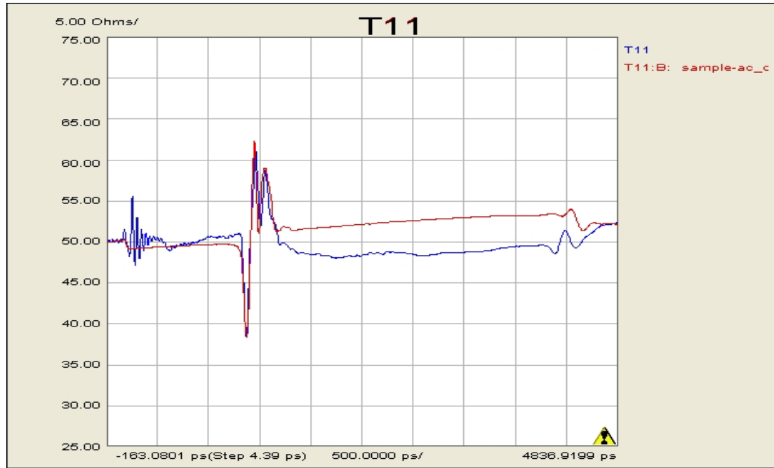
Figure 1: Measured and Simulated Z(t) Short Path.
