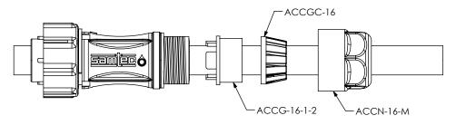
**IN-PROCESS 3** FEED SBWC-16-XX-O BUNDLED CABLE THROUGH ACCN-16-M, ACCGC-16, ACCG-16-1-2, & ACCFS-16-M-X)
