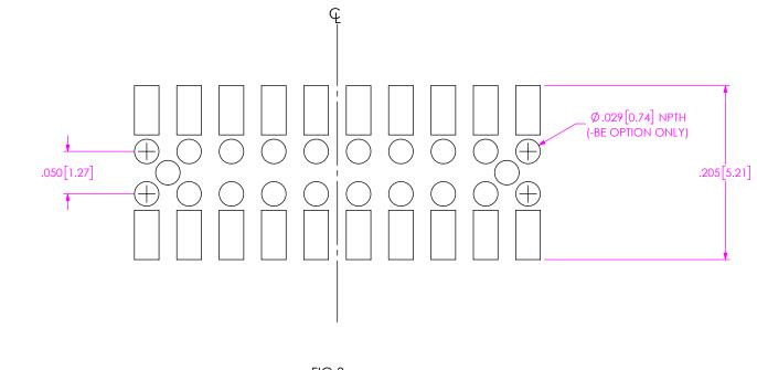
FIG 3 CLP-1XX-XX-XX-D-BE-A SHOWN SAME AS FIG 1, DIFFERENT AS SHOWN ALL DIMENSIONS ARE SYMMETRIC ABOUT THE CENTERLINE
