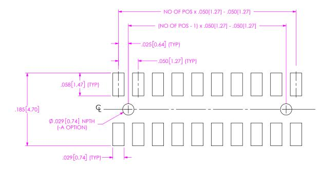
FIG 1 CLP-1XX-XX-D-A SHOWN ALL DIMENSIONS ARE SYMMETRIC ABOUT THE CENTERLINE
