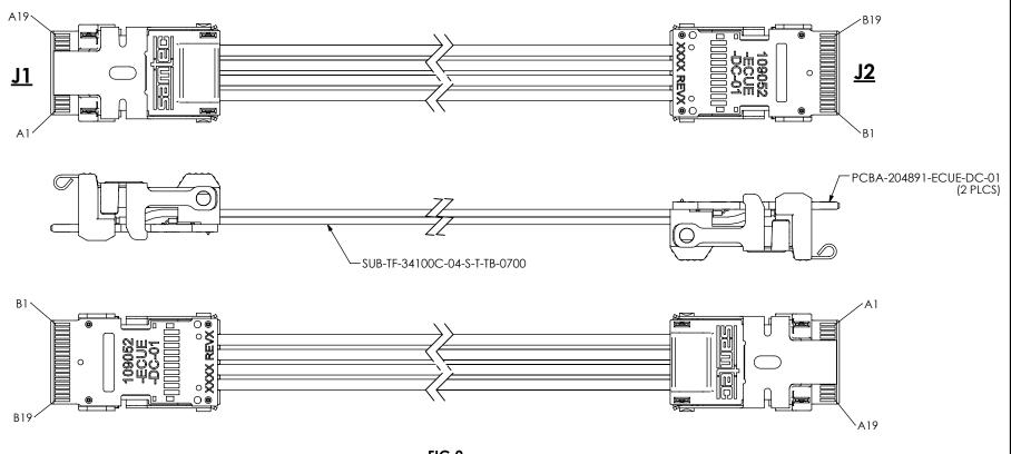
FIG 2 WIRING OPTION -02 ECUE-08-XXX-T3-FF-02-2-D1 SHOWN (DIFFERENT AS SHOWN, OTHERWISE SAME AS FIG 1)
