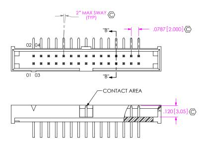
FIG 2 ETMM-115-02-X-D-RA SHOWN (DIFFERENT AS SHOWN, OTHERWISE SAME AS FIG 1)
