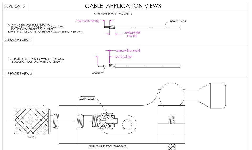
3A. THREAD PCI ASSEMBLY TOOL 450234 INTO SUHNER BASE. THEN THREAD CONNECTOR BODY ONTO PCI TOOL UNTIL SEATED.
