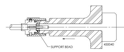
5. REMOVE CONNECTOR FROM SUHNER BASE TOOL AND INSTALL DIELECTRIC SUPPORT BEAD USING PCI TOOL SET 450040 F:\DWG\MISC\MKTG\PRF92-P-C-EE-405-SD-MKT.SLDDRW
