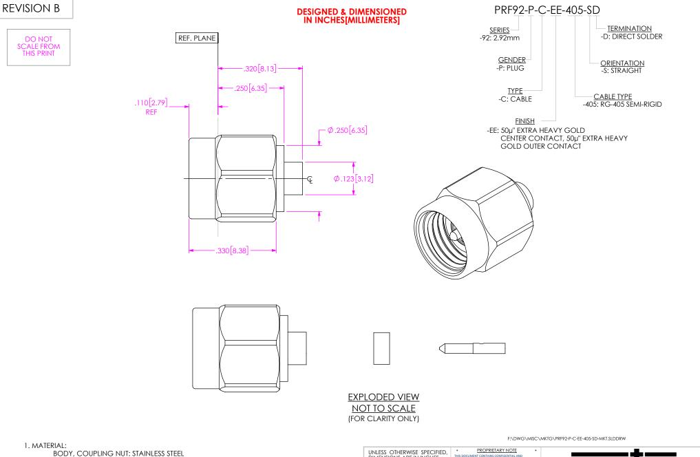
BODY, COUPLING NUT: STAINLESS STEEL CONTACT, LOCK RING: BERYLLIUM COPPER BEAD: PPE
