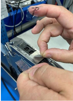
Prepare splice by taking extra scrap/new cover tape to create your leader. This is done by peeling off enough length to allow for ESD tape to create a splice between the two pieces of cover tape.
