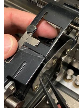
Prepare splice by taking extra scrap/new cover tape to create your leader. This is done by peeling off enough length to allow for ESD tape to create a splice between the two pieces of cover tape.
