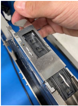
Load cut tape into feeder. (Shown) ASM load from the front and Juki loads from the back engaging the gears.
