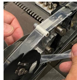
Prepare splice by taking extra scrap/new cover tape to create your leader. This is done by peeling off enough length to allow for ESD tape to create a splice between the two pieces of cover tape.
