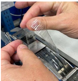
Load cut tape into feeder. (Shown) ASM load from the front and Juki loads from the back engaging the gears.
