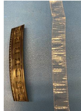
Locate scrap or extra cover tape matching the size of the feeder. 24 mm shown.
