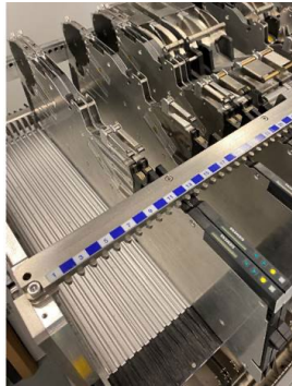
Locate Feeder Size/Style Examples shown are ASM SIPLACE SmartFeeder Electronic or JUKI Mechanical
