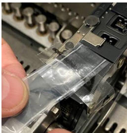
Prepare splice by taking extra scrap/new cover tape to create your leader. This is done by peeling off enough length to allow for ESD tape to create a splice between the two pieces of cover tape.
