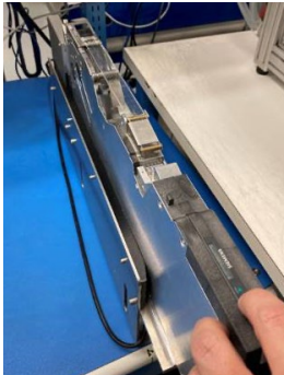
Remove slack from cover tape and tighten tension
