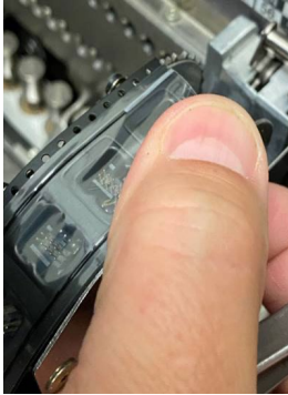
Load cut tape into feeder. (Shown) ASM load from the front and Juki loads from the back engaging the gears.
