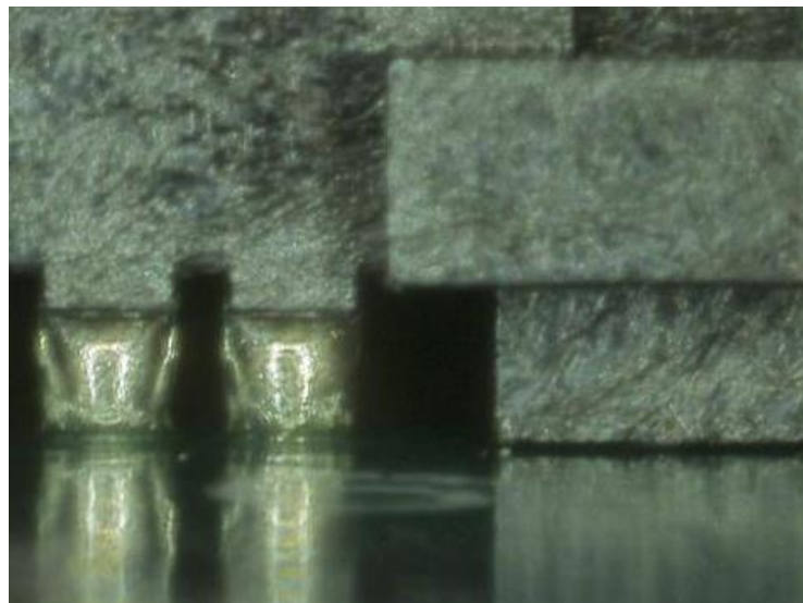
Fig. 5. The insulator housing of a reflowed SEAX8 connector will rest on the board surface or slightly above.
