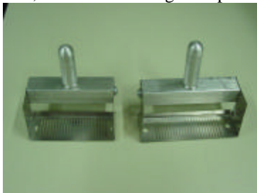
Figure 7; Mini Stencil Plug/Receptacle for Repair (6 mil)
