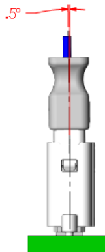
FINAL X AXIS ANGULAR MISALIGNMENT
