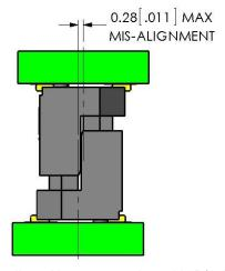
**7.1.2** The parts can be rigidly misaligned by no more than .002" (0,05 mm) in the X- and .002" (0,05 mm) in the Y-direction to ensure a good mate.
