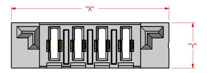
**7.1.3** For PESC / PETC, the parts can be rigidly misaligned by no more than .003" (0,08 mm) in the X-and .003" (0,08 mm) in the Y-direction to ensure a good mate.
