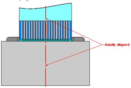
**5.1.2** Cable must be fully inserted to connector before closing the cam.
