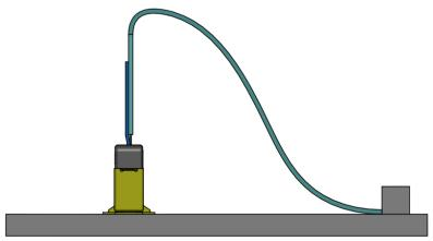
**5.1.7** The minimum bend radius is R0.16 [.006]. We recommend that the cable should not be bent in the vicinity of the stiffener. If it is bent in this area, there is a potential to cause the leads to break/delaminate and cause interruption to the signal.
