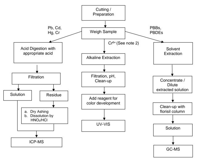
Note: 1. The Cr, Cd, Pb and Hg contents test on polymeric samples were dissolved totally by preconditioning method according to above flow chart.
