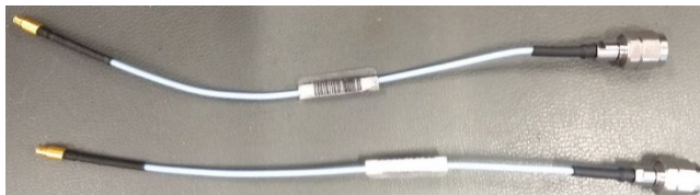
Cable assemblies used for isolation testing
