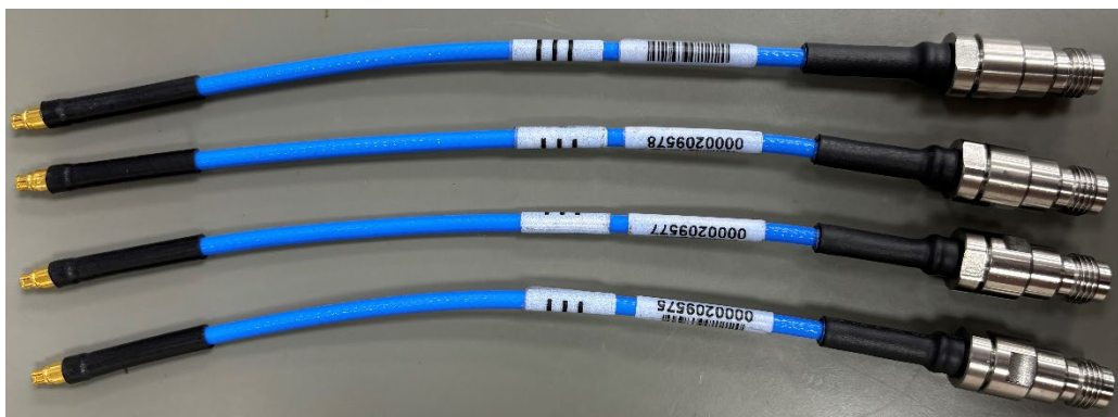
Cable assemblies used for isolation testing
