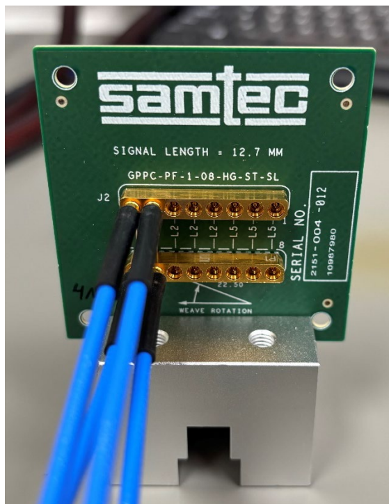
Isolation testing setup
