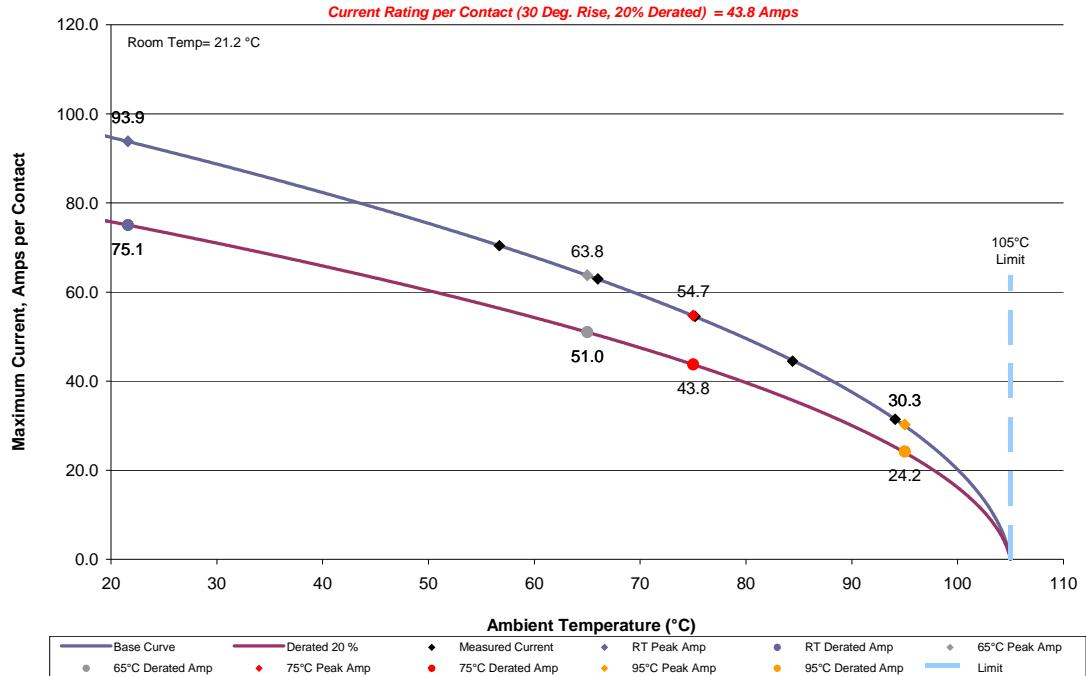
218435 (Signal Pins powered at 1/2 Rated Current)(1.05 Amps)
