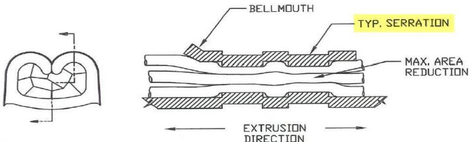
\*\* Examine for compliance with PASS/FAIL criteria: No broken/missed wires, voids, cracks in the contact material or other applicable defects shall be allowed.
