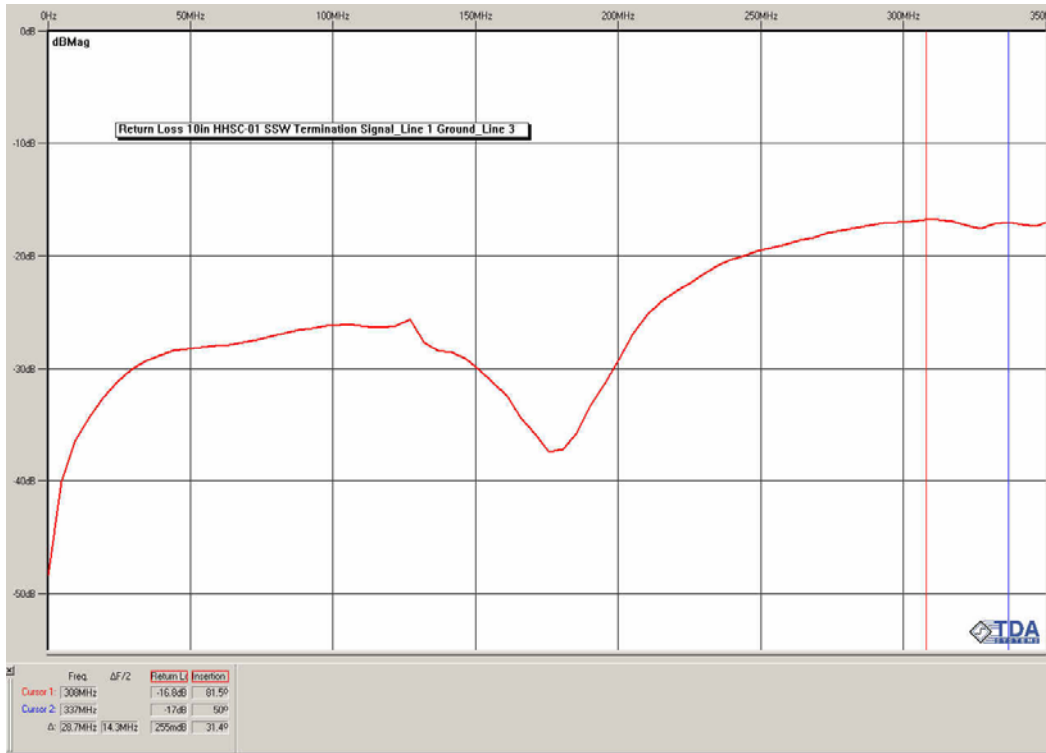
Figure 6: HHSC-108-10.00-SU-TD; Return Loss, Signal Line 1, Ground Line 3
