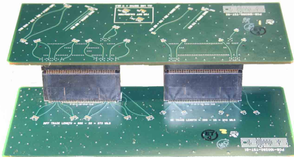
Figure 1 Mated PCB Test Fixture with Mounted Test Connectors
