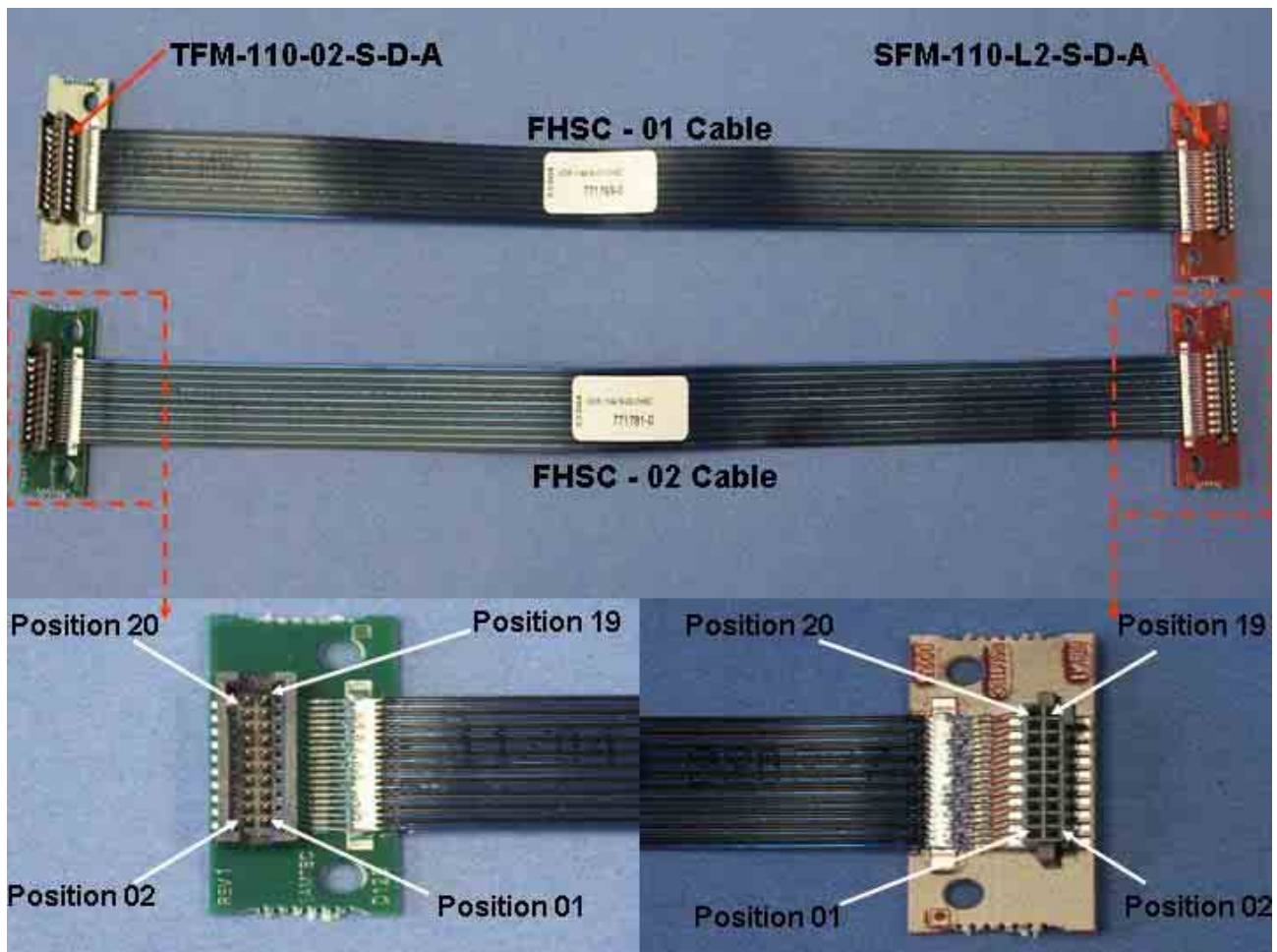
Figure 1: 10.00" FHSC-01 and FHSC-02 Cable Assembly. Shown with caps off.
