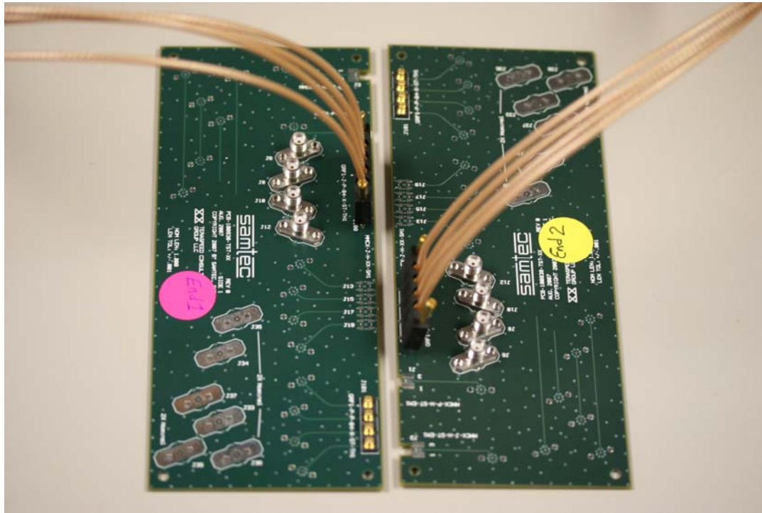
Figure 14: Test setup with Test PCBs and GRF1-C cable.
