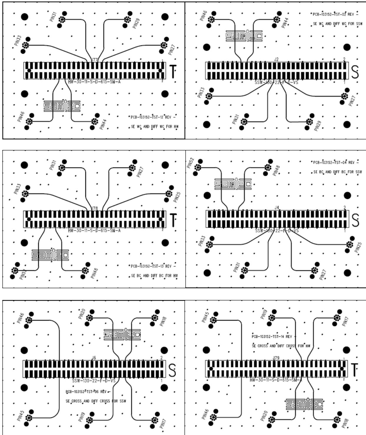
**Series:** HW/ SSW**Description:** High Temperature Board Stacker, 0.64mm (.025") Square Post, Surface Mount Terminal Strip, 0.100" [2.54mm] Pitch, 25.4mm (1.000") Stack Height**Calibration Board**
