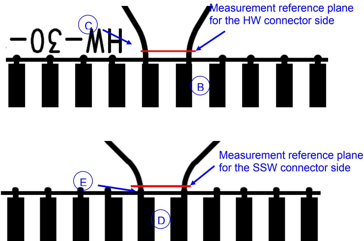
**Series:** HW/ SSW**Description:** High Temperature Board Stacker, 0.64mm (.025") Square Post, Surface Mount Terminal Strip, 0.100" [2.54mm] Pitch, 25.4mm (1.000") Stack Height
