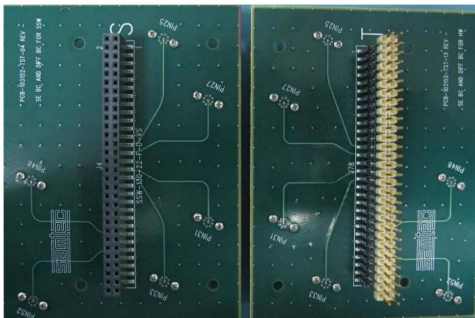
**Series:** HW/ SSW**Description:** High Temperature Board Stacker, 0.64mm (.025") Square Post, Surface Mount Terminal Strip, 0.100" [2.54mm] Pitch, 25.4mm (1.000") Stack Height**PCB-103152-TST-XX PCB Layout Panel**
